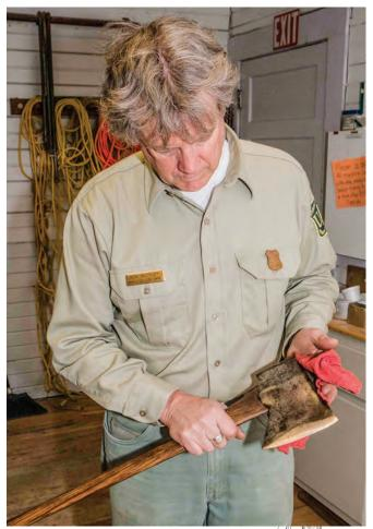
Figure 12–2—Cleaning an ax head with a rag.
