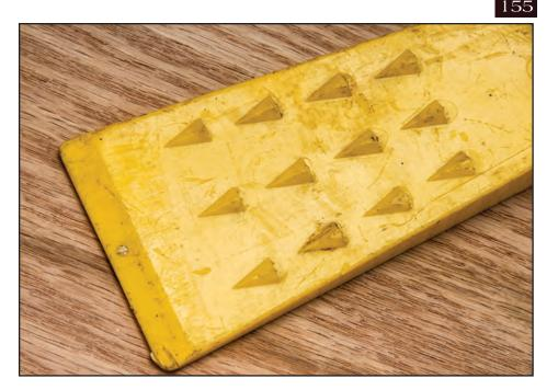
Figure 11–54—A wedge with a ridged surface.
