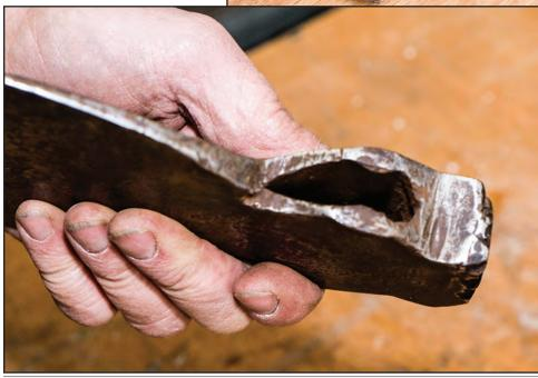
Figure 13–8 – Distortion around the bottom of an L&IJ White broad hatchet head eye. This kind of damage usually occurs when someone tries to remove a handle using a hammer.
