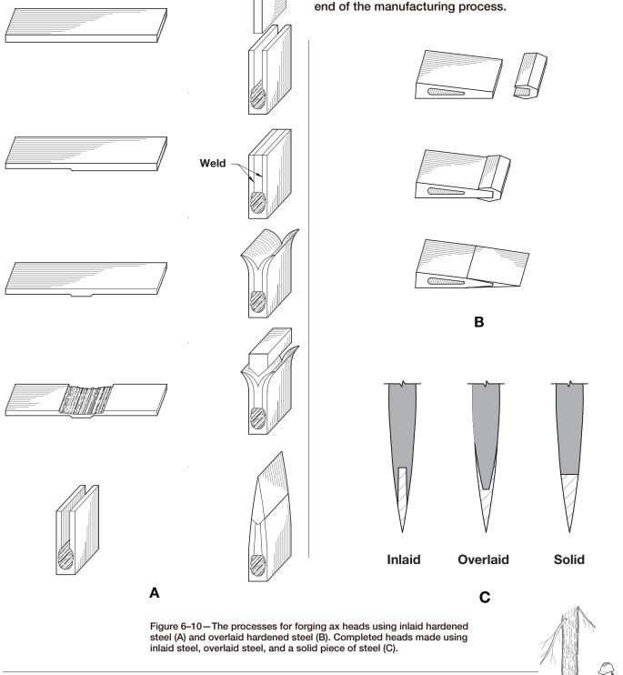
The hardened (tempered) cutting edges were durable and long-lasting. The softer center mass of the ax also provided an important feature: as the hardened steel cutting edge sank into a piece of wood, it transferred the shock of the blow into the ax head (figure 6–11). When the shock reached the cheeks of the ax, the softer metal helped absorb and dissipate the energy, reducing the amount of shock that transferred down the handle and into the axman's hands.
