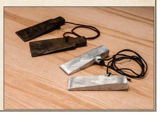
Figure 11–56—Newly manufactured aluminum holding wedges (foreground) tend to be thicker than vintage holding wedges (background).
