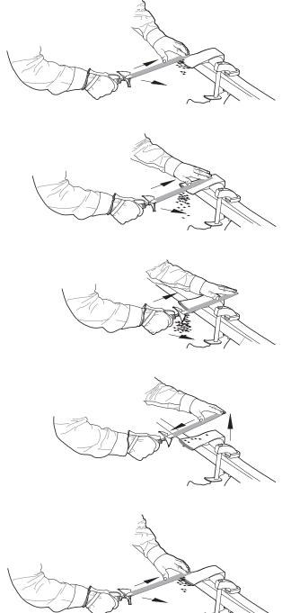
Figure 7–5–Push filing, showing the forward motion.
