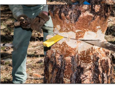
Figure 11–45–Placing a wedge lightly in the kerf of the tree will help alert you when the tree begins to fall.
