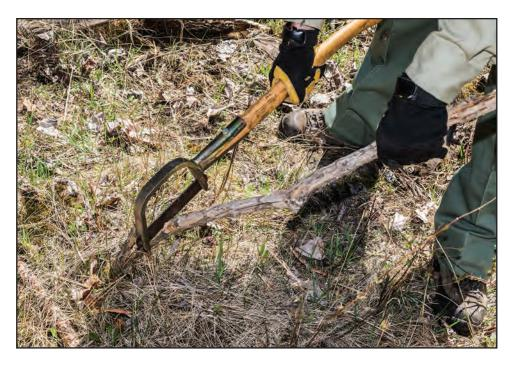
Figure 11–29–Using a Swede ax to cut a dead sapling.
