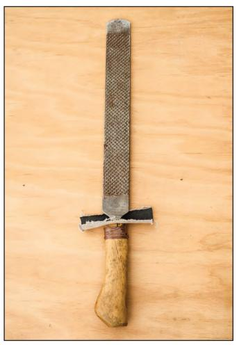
Figure 7–4–A rasp (the author used a broken ax handle to make a handle for this rasp).
