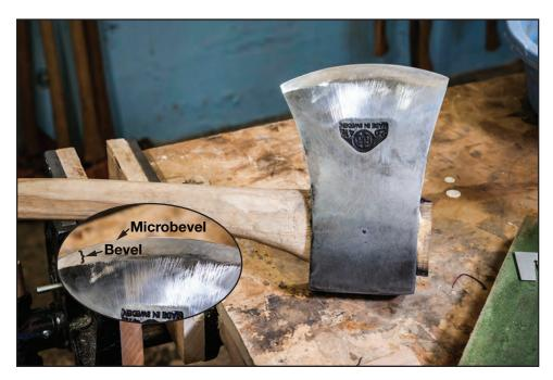
Figure 8–2—The microbevel in relation to the bevel. The inset shows a closeup view of the microbevel and bevel.
