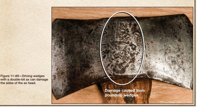
When splitting wood, the cutting edge of an ax head should be sharp, and the sides should be thicker. This enables the ax to have greater splitting action once the cutting edge penetrates the wood. The longer handle enables you to generate more speed as you swing the ax.
