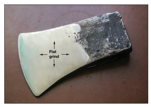
Figure 8–16—A flat grind on a flatprofiled ax.
