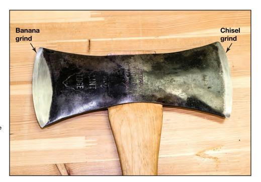
Figure 8–15—A double-bit ax with a banana grind on one cutting edge and a chisel grind on the other.
