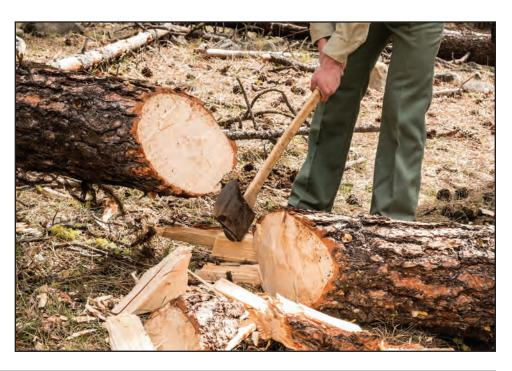
Figure 11–32—Using the poll of an ax to break through a log.
