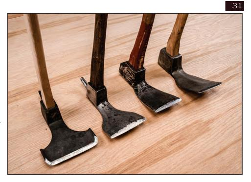
Figure 5–26 – Various adzes (right) – note the differences in curvature of each blade – and a gutter adz and bowl adz (below).
