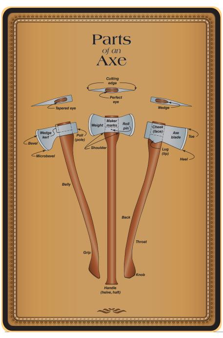
Figure 4–1—Pats of single- and doublebit axes. Refer to "Appendix A—Full-Page Ax Illustrations" for a larger version of this illustration.
