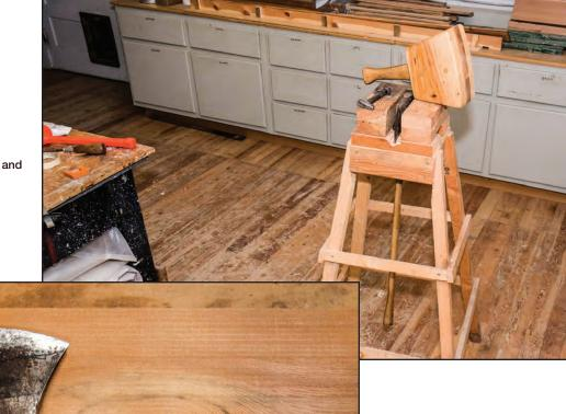
Figure 10–5–A jig, drift, and wooden mallet.
