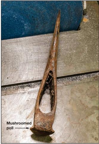
Figure 13–16—The photo above shows major mushrooming on a poll. The top photo on the following page shows someone grinding down the poll using a disc sander. The bottom photo on the following page shows the reshaped (reprofiled) poll.
