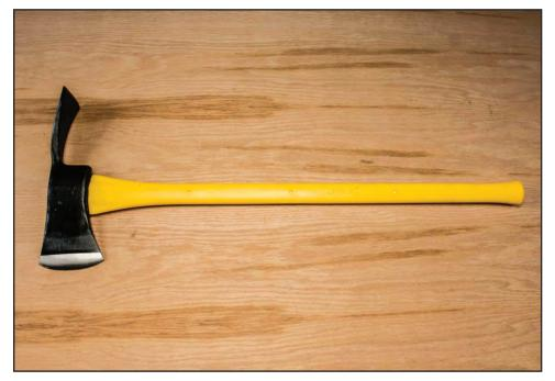
Figure 6–13—A pulaski with a synthetic handle.
