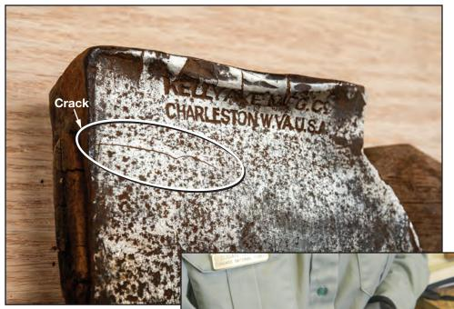
Figure 8–21 – A crack in an ax head. When you see a mushroomed poll, check carefully around the eye for cracks.
