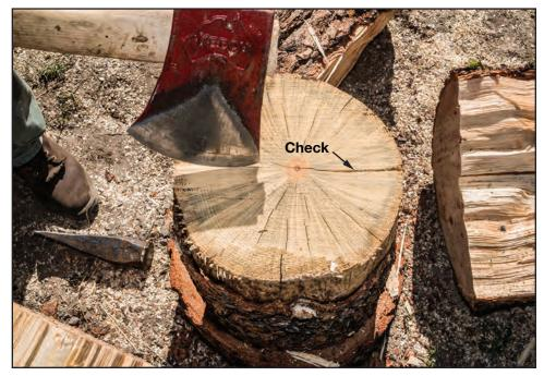
Figure 11-72-Use splits or checks in the wood when splitting a round of wood with an ax.
