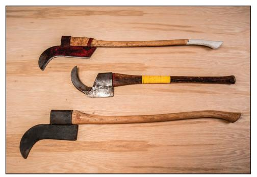
Figure 5–18 – Three brush axes.
