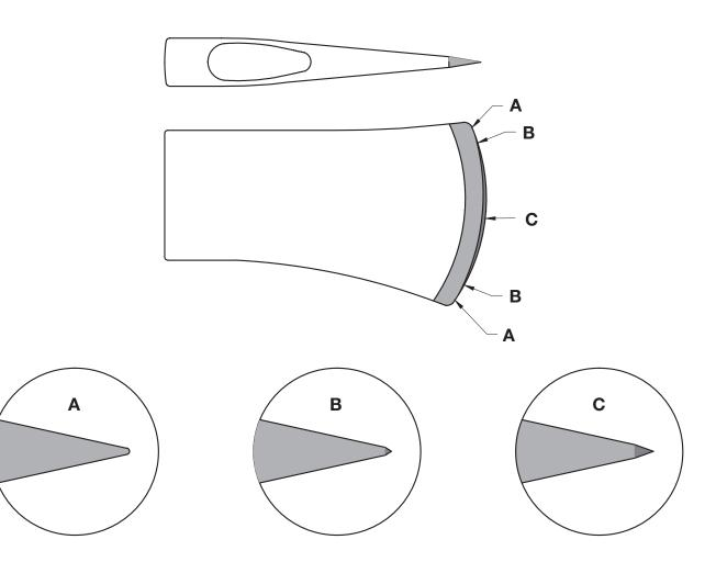
Figure 8–28—The ends of the ax head (the toe and heel) are unsupported edges. Leave the toe and heel slightly thicker to prevent the cutting edge from chipping.
