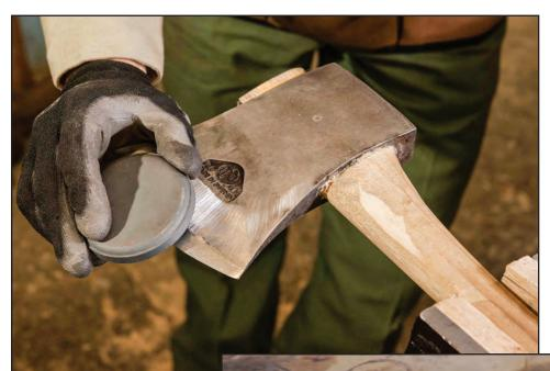
Figure 8–31 – Using an ax stone to hone the bevel.
