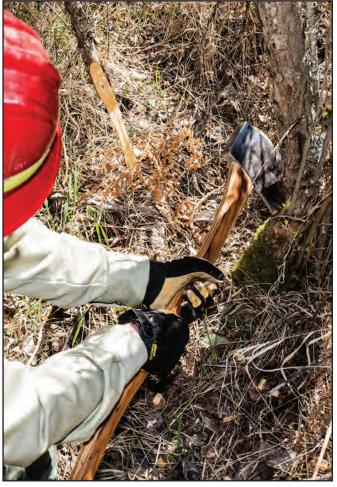
Figure 11–27—A choked grip makes it easier to cut brush, though there may be other tools that are more appropriate for the job, such as lopping shears or a small pruning saw.
