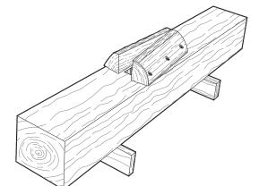
WOOD GUIDES CAN BE SCREWED INTO POST AT AN ANGLE TO HOLD AXE HEAD SECURE.
