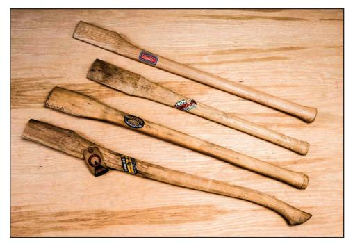
Figure 6–1 – Unused old stock ax handle blanks.
