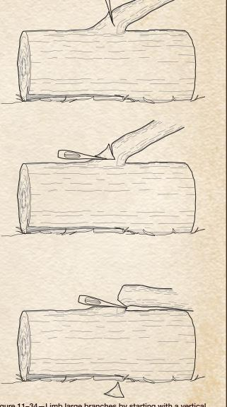
Figure 11–34—Limb large branches by starting with a vertical chop. Follow this with a horizontal chop to remove a wood chip.
