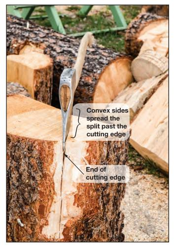
Figure 8–12—A convex head in a round of wood. Note that the sides of the ax head spread the round apart well beyond the cutting edge.
