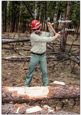
Figure 11–17—Holding an ax with one hand on the throat and the other hand on the shoulder.
