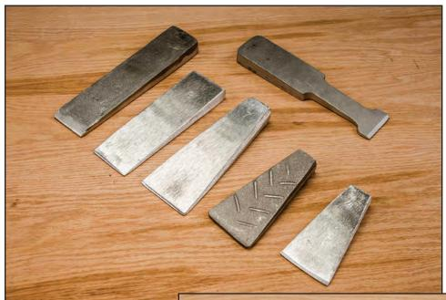
Figure 11–52—Aluminum wedges.
