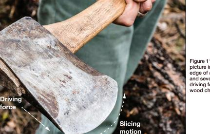
Figure 11–13—The arrows in this picture indicate how the cutting edge of an ax head slices through and severs wood fibers and how the driving force helps to pop out the wood chip.
