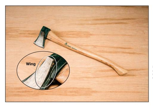
Figure 11–71 – A modern splitting ax with wings that help spread and split the log. The inset shows a closeup of one wing.
