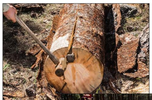
Figure 11–79—Using a sledge hammer and wedge to split a rail from a log.
