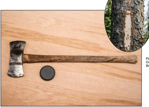
Figure 5–15–A Shapleigh Hardware Company Diamond Edge saddle (blazing) ax.
