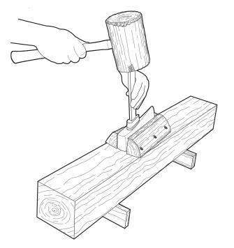
CUT OFF HANDLE. USE DRIFT PIN AND HAMMER TO DRIVE REMAINING HANDLE FROM BOTTOM OF EYE THROUGH TOP OF EYE.
