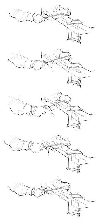
Figure 7–6–Draw filing, showing the lateral motion.
