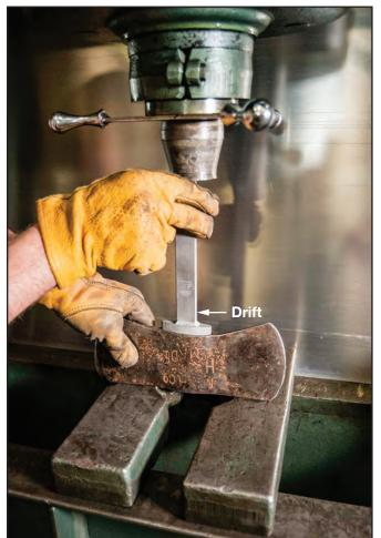
Figure 3–15–Using a drift pin to reshape an ax head eye.
