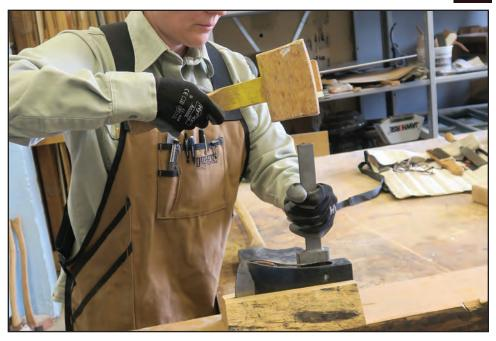
Figure 9–4—Using a mallet and drift pin to remove the remaining portion of a handle from an ax head eye.
