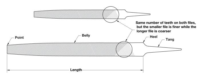
Figure 7–2–Swiss files are measured from the point to the heel.
