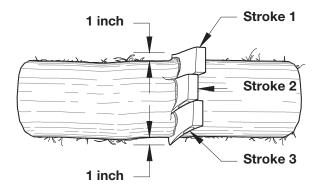
Figure 11–31—Chopping the top of a log lying horizontally. The first stroke chops the far side of the log; the second stroke chops the center of the log, overlapping the first stroke; and the third stroke chops the near side of the log, overlapping the second stroke.
