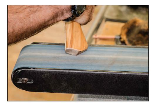
Continue rasping and seating the handle until the head fits snuggly on the shoulder. Each time you place the ax head, sight down the cutting edge to ensure that it stays laterally aligned with the knob of the handle (see figure 10–3). If the alignment is to the right, remove wood from the right side of the handle that sits inside the eye (figure 10–11). If the alignment
