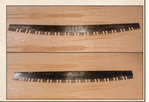
Figure 11–46—A felling saw (top) and a bucking saw (bottom).
