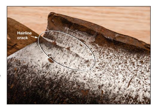
Figure 13–9–A hairline crack in an ax head.
