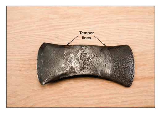
Figure 13–3 – Temper lines on a 1933 Sager Chemical double-bit ax head. Note the pitting in the softer metal at the center of the head. Despite the pitting, this ax has ample hardened steel on both cutting edges and can be restored to a good working ax.
