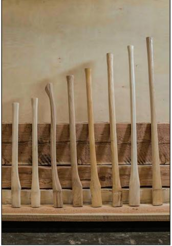
Figure 11-26 – Various sizes of ax handle, ranging from 26 inches to 44 inches.
