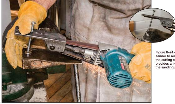
Figure 8–24—Using an electric sander to remove metal from behind the cutting edge. A rare earth magnet provides an excellent pivot point for the sanding jig (inset).
