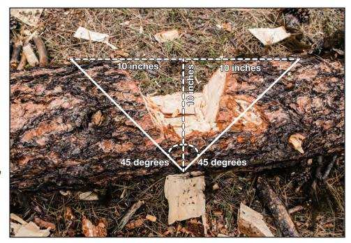
Figure 11-21 — This notch is too narrow to continue removing big chips; it must be wider to enable the ax to cut through to the bottom of the log.
