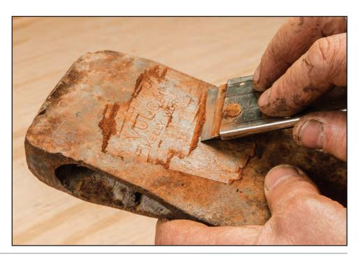
Figure 13–11 – Using a razor blade scraper to remove rust from an ax head.
