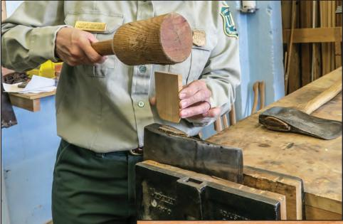
Figure 12–6 – Using a new, thick wooden wedge and a mallet to tighten a loose ax head.
