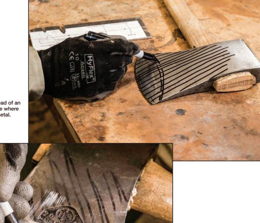
Figure 8–4 – Marking the head of an ax with a felt pen to indicate where and where not to remove metal.
