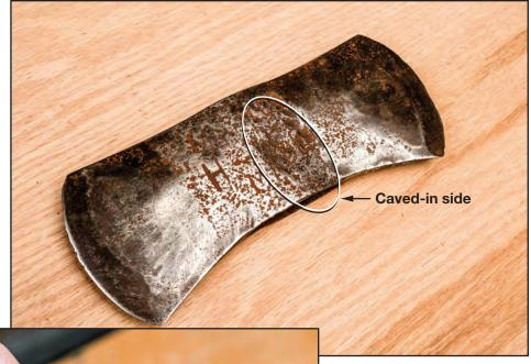
Figure 13–7 – The eye of this Marshall Wells double-bit ax has caved-in sides.
