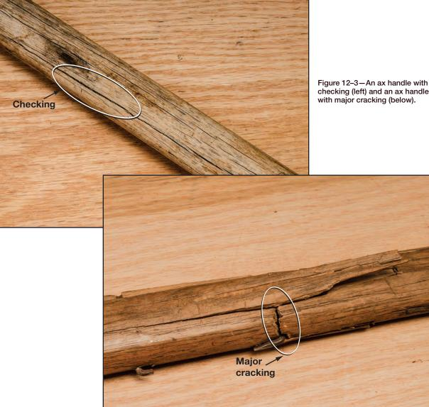
checking (left) and an ax handle with major cracking (below).
