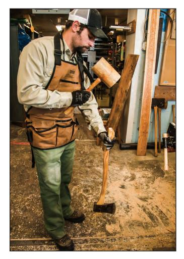
Figure 10–9—Strike the heel of the ax handle to draw the ax head onto the handle. Note that the fawn's foot on this handle has a flat bottom.
