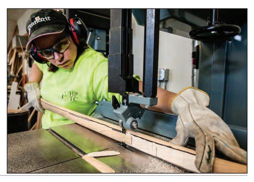
Figure 9–7–Using a band saw to thin down a thick handle.
