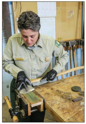
Figure 8–34 – Using a leather strop to sharpen a cutting edge.
