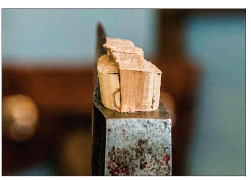
Figure 10–17 – The wedge expands the top portion of the ax handle to grip the sides of the ax head eye.
