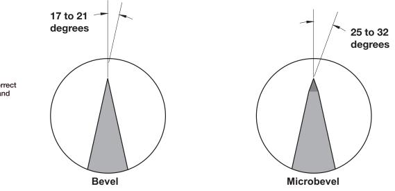
Figure 8–3 – The correct angles for a bevel and microbevel.
